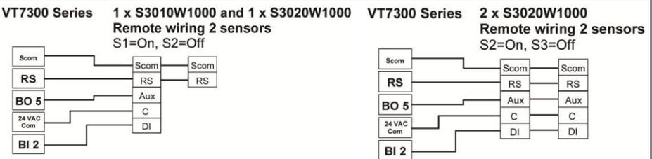
**VT7300 Series 2 x S3010W1000 Remote wiring 2 sensors**
